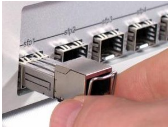
Figure 2.4. Installing a 1000 Base TX module
